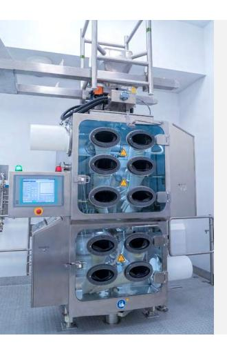
Roller compaction turns powder blends into densified sheets using the pressure of two compacting rollers. The resulting sheets can then be milled to any desired mesh size providing an efficient and scalable process. PCI has invested in contained Gerteis Mini-Pactor technology to further expand our contained manufacturing operations. This technology offers a patented proven design able to process highly potent molecules using effective containment technology and integrated cleaning systems.
